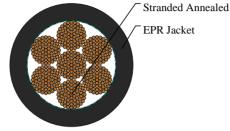
Stranded Annealed Copper Conductor
